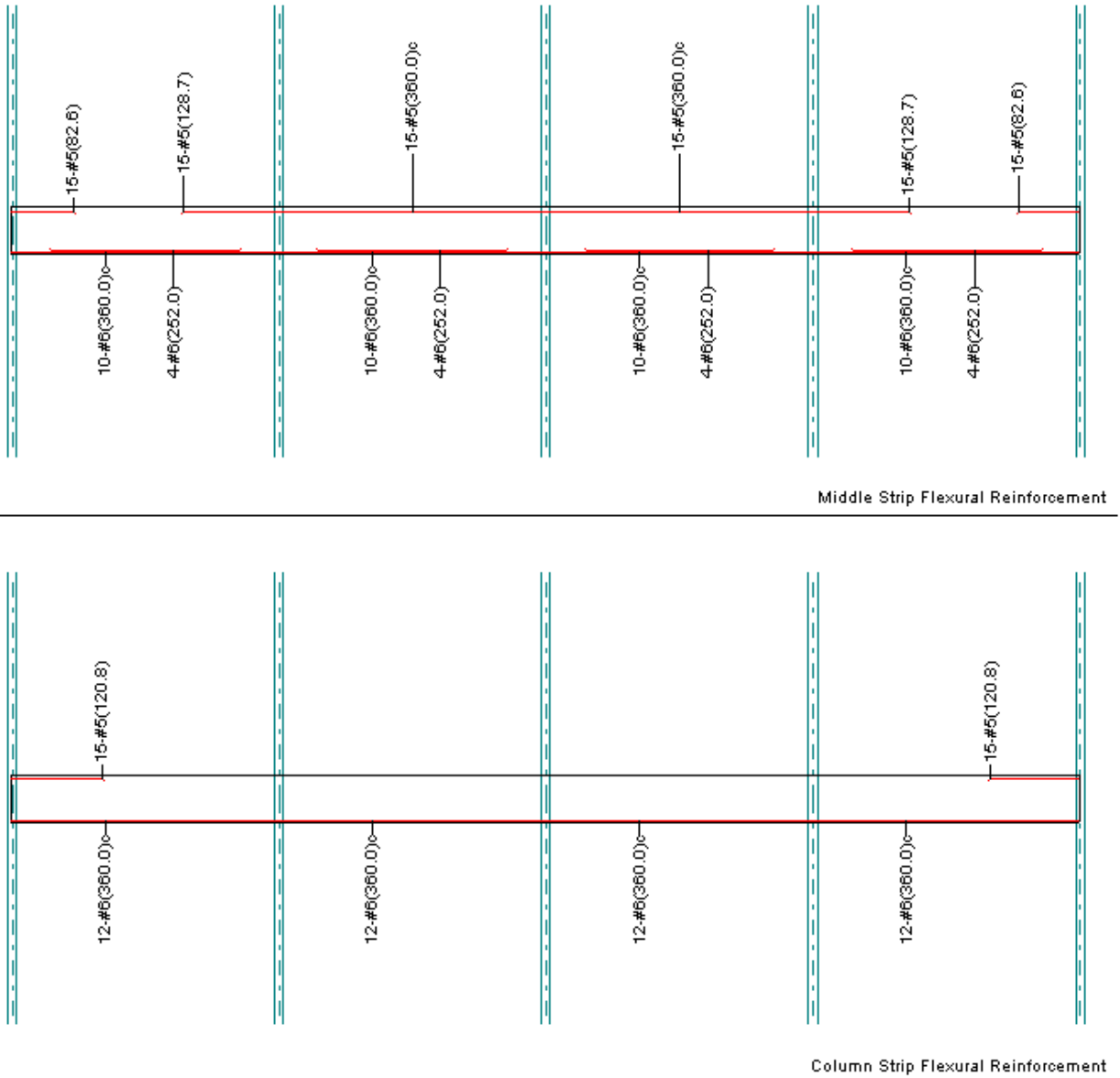
Figure 31 – Waffle Slab Reinforcing Design
