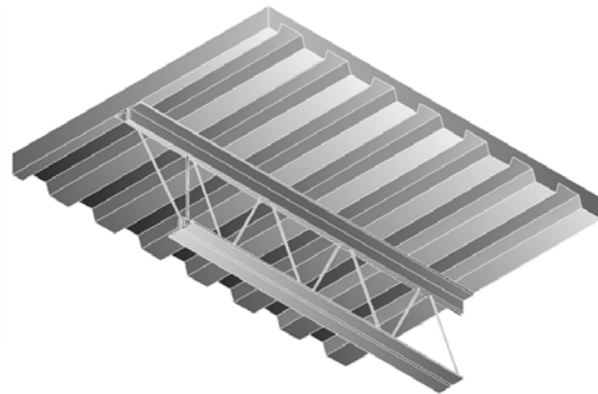
Figure ??? – Joist and Slab System
