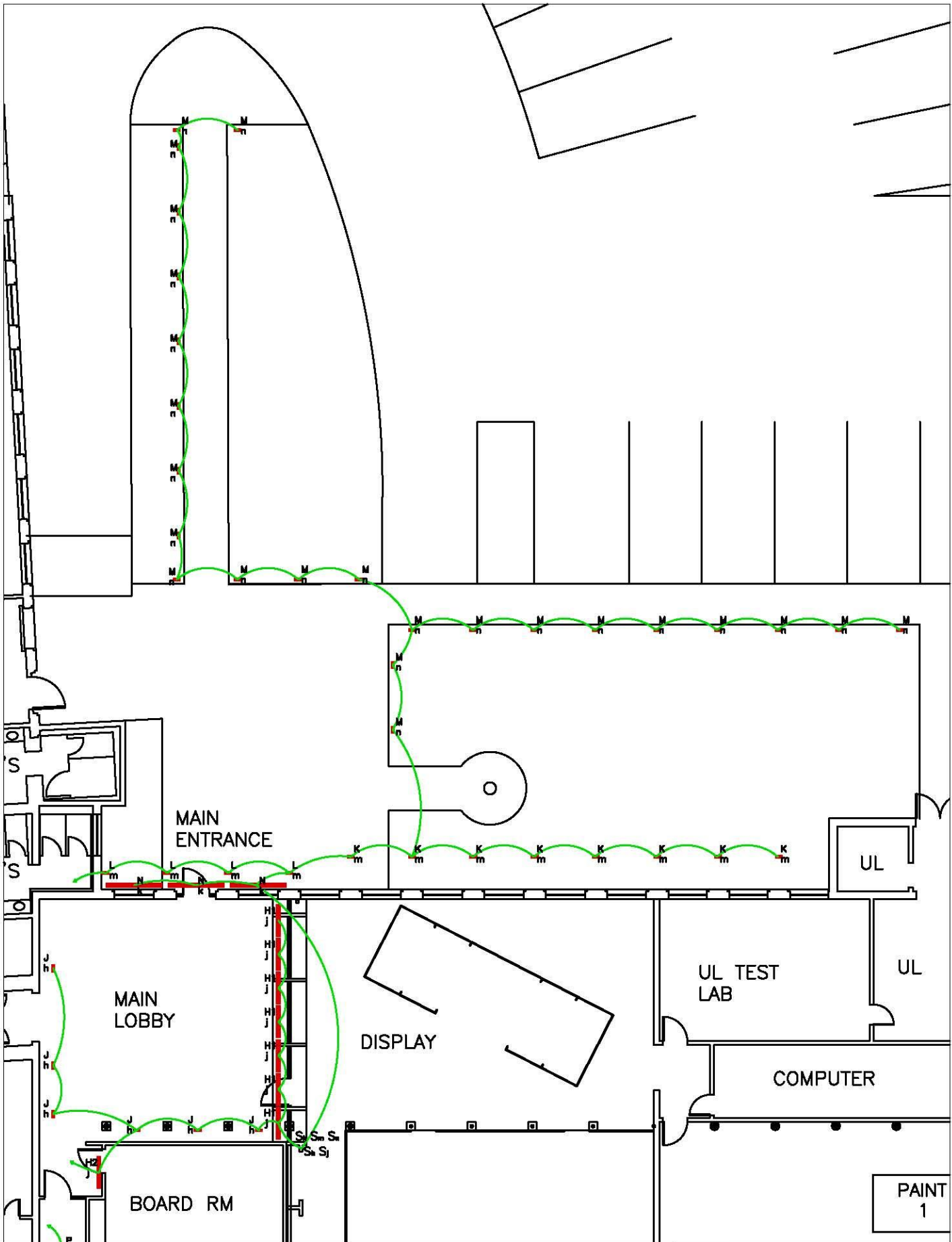
APPENDIX A LIGHTING PLAN MAIN ENTRANCE SCALE: 1/16"=1'-0"
