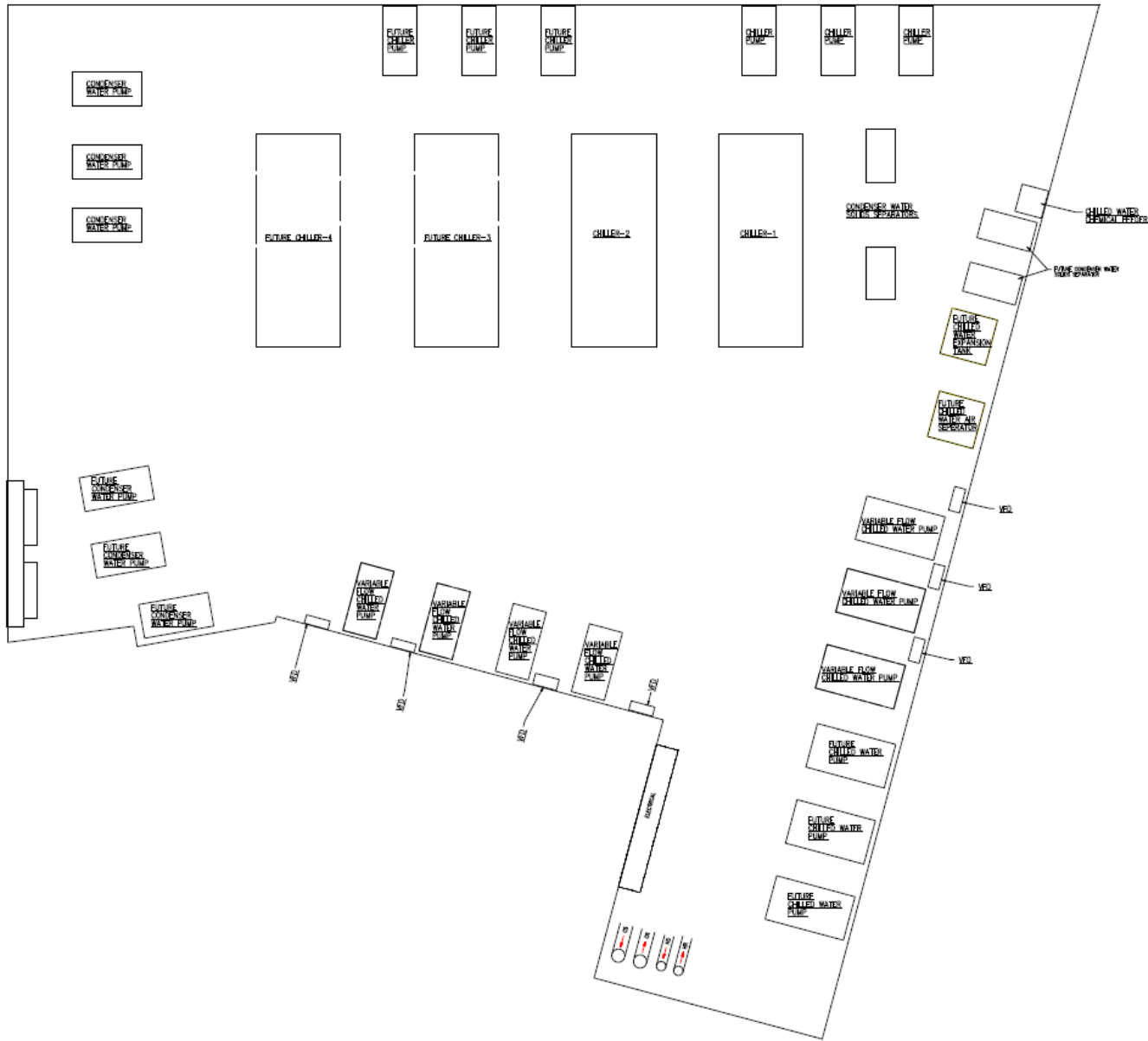
Figure 12 – Simplified Cooling Central Utility Plant
