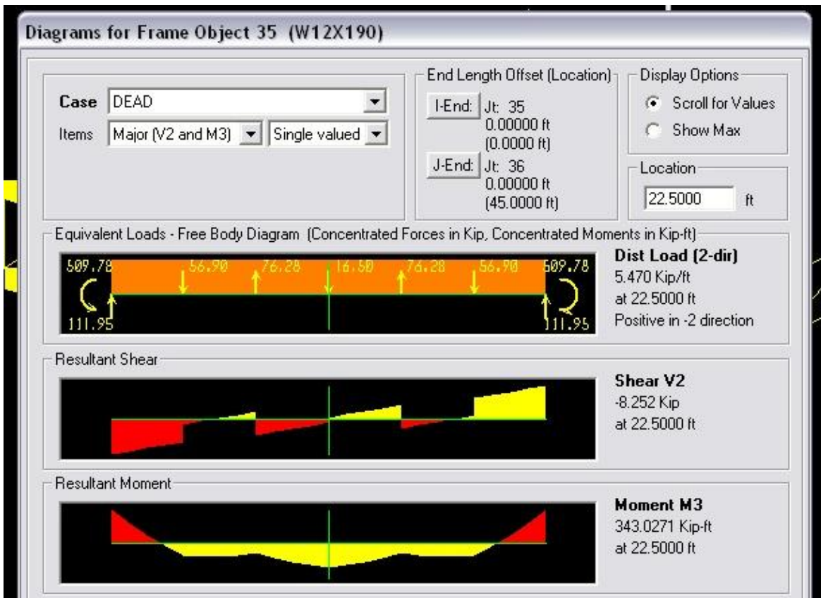
Figure 39: SAP Model of Top Cord Shear and Moment
