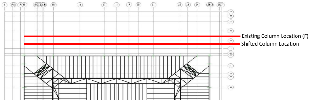
Figure 18: (Above) Typical corner column impact on surrounding structure at Club (Top) and Concourse (Bottom) levels.
