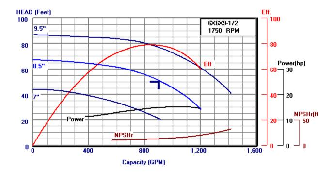
Pump Series: 80 Min Imp Dia = 7 " Design Capacity = 900.0 ITT Bell & Gossett
