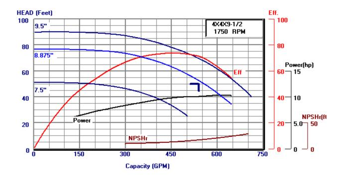
Pump Series: 80 Min Imp Dia = 7.5 " Design Capacity = 540.0 ITT Bell & Gossett Suction Size = 4 " Max Imp Dia = 9.5 " Design Head = 50.0 Motor Size = 10 HP Morton Grove, II 60053
