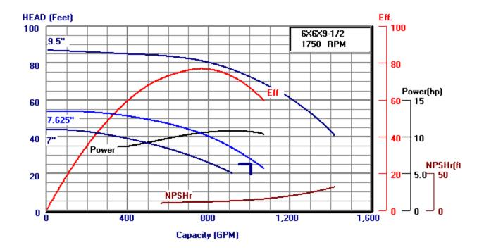
Pump Series: 80 Min Imp Dia = 7 " Design Capacity = 1008.0 ITT Bell & Gossett
