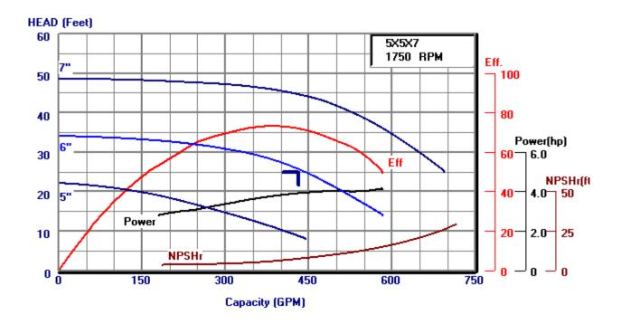
Pump Series: 80 Min Imp Dia = 5 " Design Capacity = 432.0 ITT Bell & Gossett Suction Size = 5 " Max Imp Dia = 7 " Design Head = 25.0 8200 N. Austin Morton Grove, II 60053
