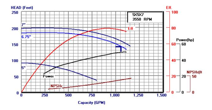
Pump Series: 80 Min Imp Dia = 5 " Design Capacity = 1055.0 ITT Bell & Gossett
