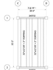
The design requires 12' wide by 32" deep double-tee beams and 24" wide by 32" deep inverted tee girders. This system will weigh approximately 1,815,000# per floor.
