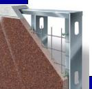
**ENVELOPE**—Traditional Virginian brick detail on exterior achieved through slender wall pre-cast concrete panel system, allowing 25% less themal transfer than traditional walls
