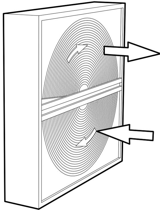
The rotor, which may be removed from the frame, is mounted in sealed permanently-lubricated spherical ball bearings. The bearings can be serviced or replaced without removing the rotor from the case.
