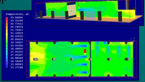
Diffuser placement & supply flow rates – acceptable!
