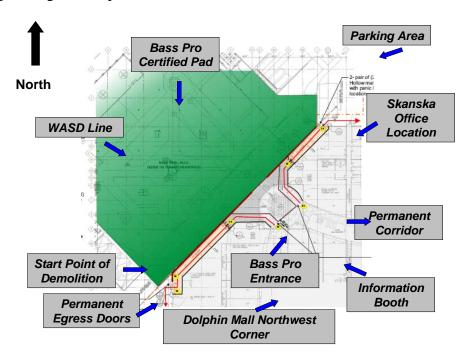
• The WASD (Water and Sewer Department) line is shown in the graphic above. This line runs directly through the Bass Pro Pad. It is the only existing utility that was not removed from the project. All storm water lines are to be installed prior to grading. The green represents the future Bass Pro Shop footprint.
