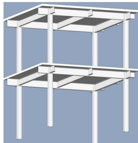
Figure 3: Model of typical steel framing layout
