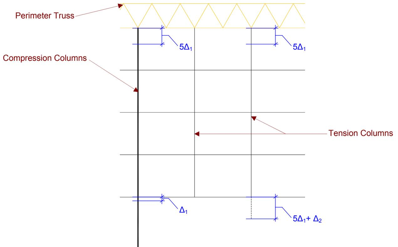
Figure 23: Column deformation
