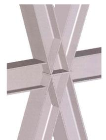
Figure 7: Diagrid connection
