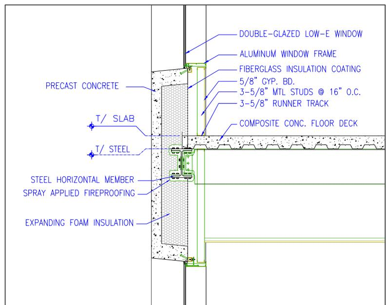
Figure 36b: Spandrel beam detail
