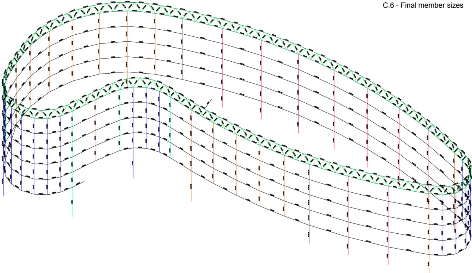
**Truss Horizontal Members - Partial Bracing**
