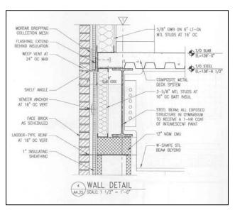
slab on metal deck (see *Wall Detail* - left). The entire brick system weighed roughly 228,800 lbs. The Slenderwall® System is supported by a connection plate that is welded to the steel angle pour stop and braced by a connection plate welded to the bottom of a steel beam (see *Typical Spandrel* detail – below right). These connection plates are to be bolted to the stainless steel framing, which is spaced at 16" O.C.
