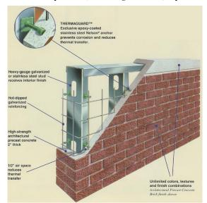
After a full analysis that addressed the impacts to cost, schedule, structural loads, and mechanical loads, the Slenderwall® is viewed to be better than the original brick face in all categories except cost. The sections on the following pages will give a detailed view of each analysis and their outcomes.
