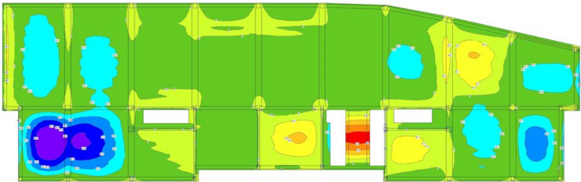
Sustained Service LC Vertical Deflection Plot
