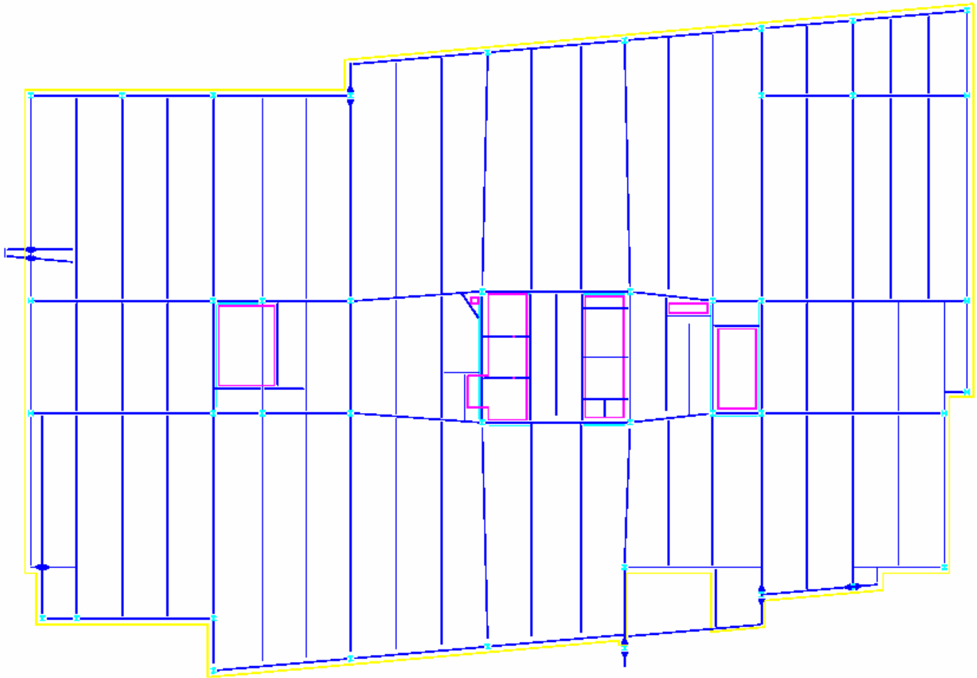
Typical Steel Framing Floor
