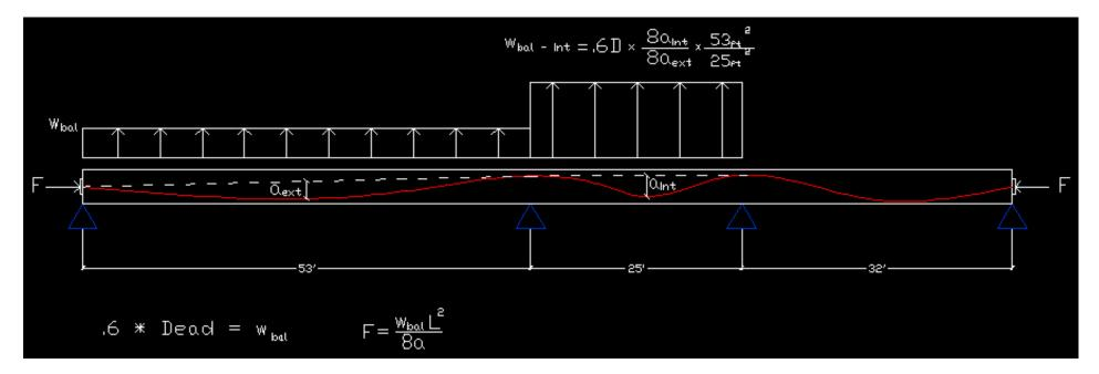
The most practical solution to preventing uplift for the middle span is to design a tendon profile that actually pushes down on the slab.
