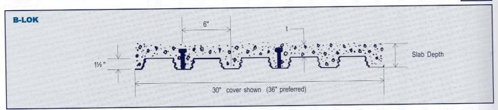
The **Deck Section Properties** are per foot of width. The I value is for positive bending (in.<sup>4</sup>); t is the gage thickness in inches; w is the weight in pounds per square foot;  $S_p$  and  $S_n$  are the section moduli for positive and negative bending (in.<sup>3</sup>);  $R_b$  and  $\varphi V_n$ . are the interior reaction and the shear in pounds (per foot of width); studs is the number of studs required per foot in order to obtain the full resisting moment,  $\varphi M_{nf}$ .
