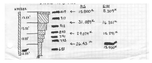
Seismic Loading, Composite Steel Structure
