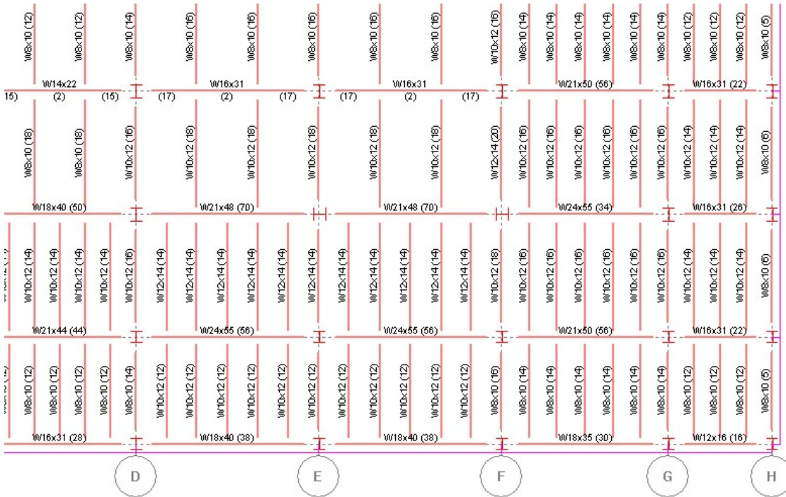
Figure 4. Basic Gravity Load Design of Parking/Driveway Surface using RAMSteel.
