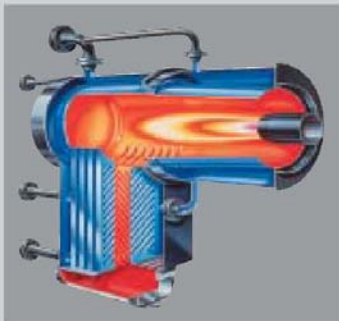
Flue gas passage within the gas-fired condensing boiler Vertomat
