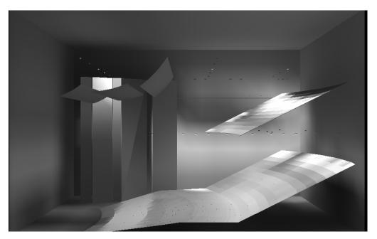
Maintenance in this space is a concern. The incandescent fixtures used above the seating area are difficult to reach by ladder or other equipment. They also need replaced frequently because of the type of source and also because they are used during set up and clean up of the space.
