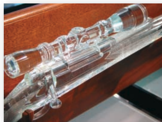
Hunting Rifle Waterjet cut and Bonded PPG Starphire that is ground and polished to a full size replica
