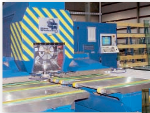
Consistent and repetitive workmanship in hole locations is provided by state of the art CNC hole drilling and milling equipment
