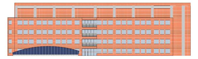
The new elevation takes many cues from the surrounding buildings. The upper level aluminum columns break up the extensive amount of blank brickwork that is needed around the 25' penthouse. The ribbon windows are broken up to reflect the traditional window pattern found in an office building. The cast stone balconies work with this traditional façade just as well as with the modern façade, and provide a look of significance for the entrance.
