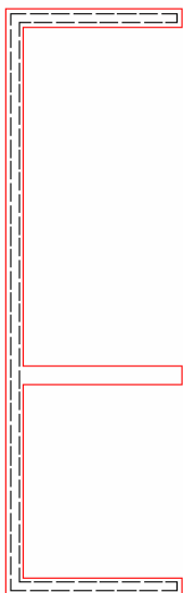
Fig. 5. Shear wall without tie beams.
