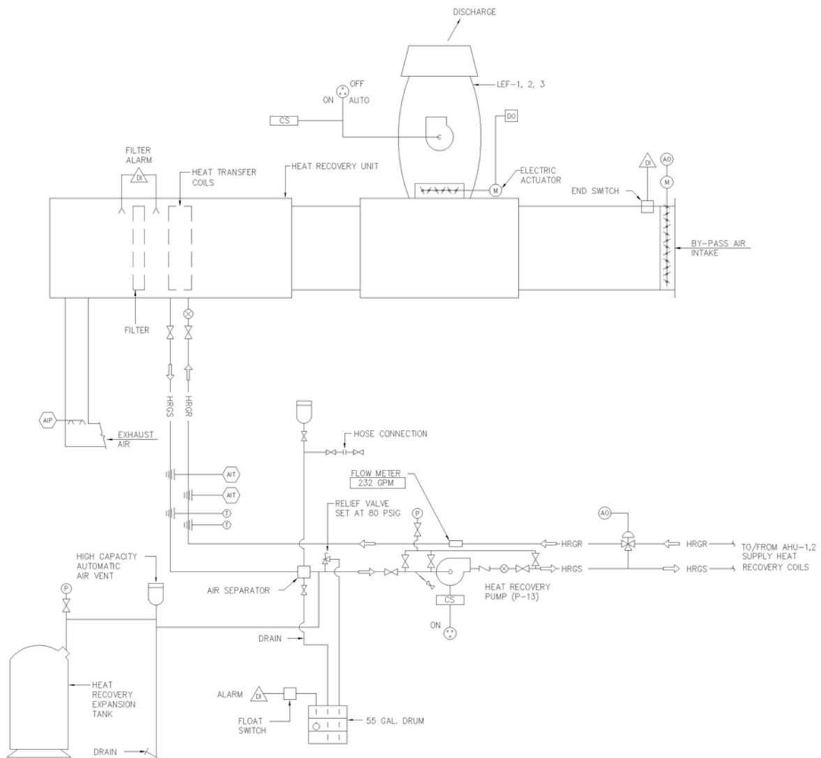
Figure XIII: AHU-1 and AHU-2 Flow and Control
