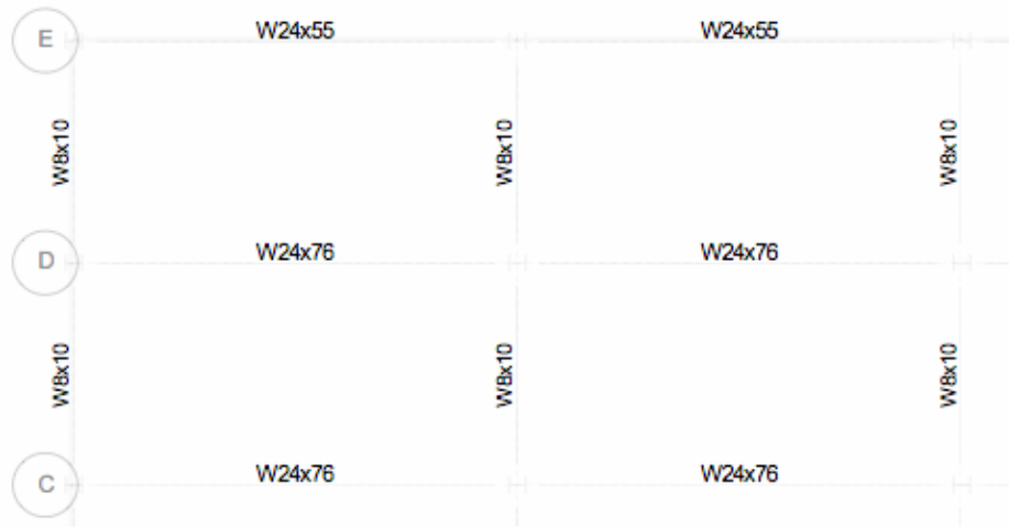
Figure 15 – Steel beam layout for P/C panels
