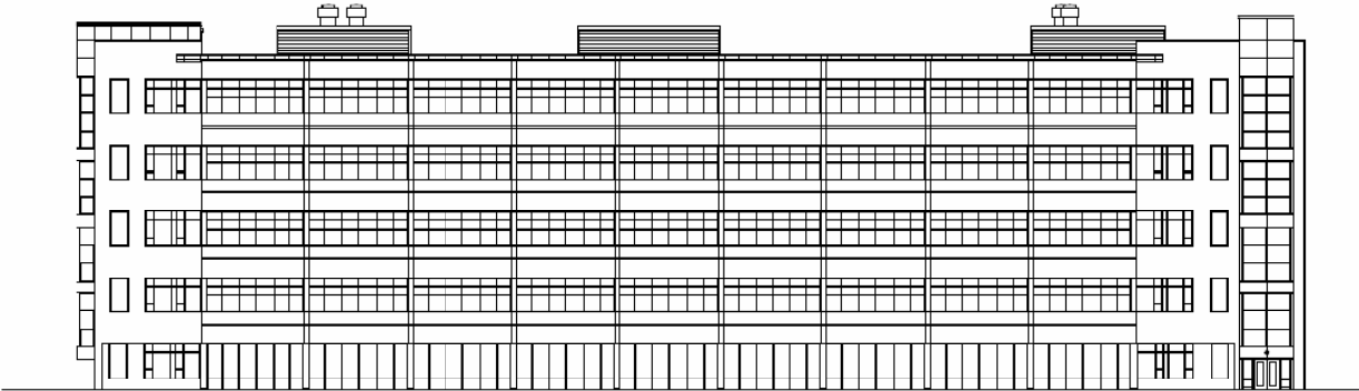
Figure 9. South Elevation of Proposed 5-story Rectangular Wing
