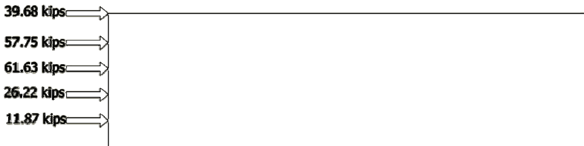
Figure 26. East-West Seismic Story Loading
