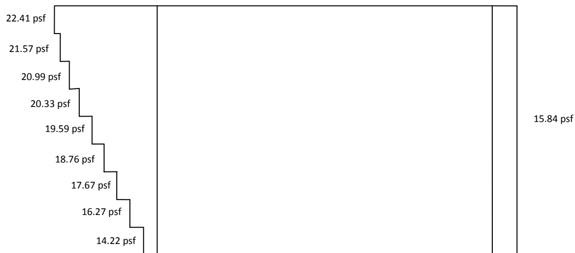
Figure 12: The Southern Building N-S Wind Loads
