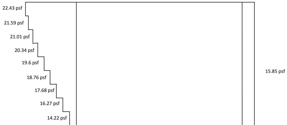
Figure 14: The Southern Building E-W Wind Loads
