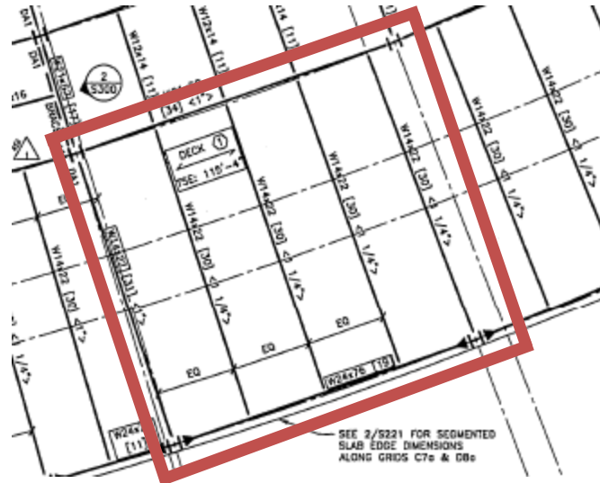
Figure 19: Typical Bay Selected for Metal Decking Spot Check
