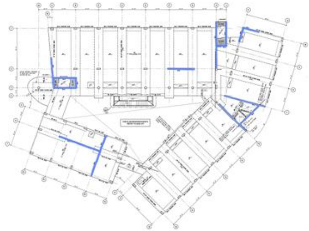
Figure 4 Typical floor plan taken from Sheet S203. Shear walls are indicated in blue.
