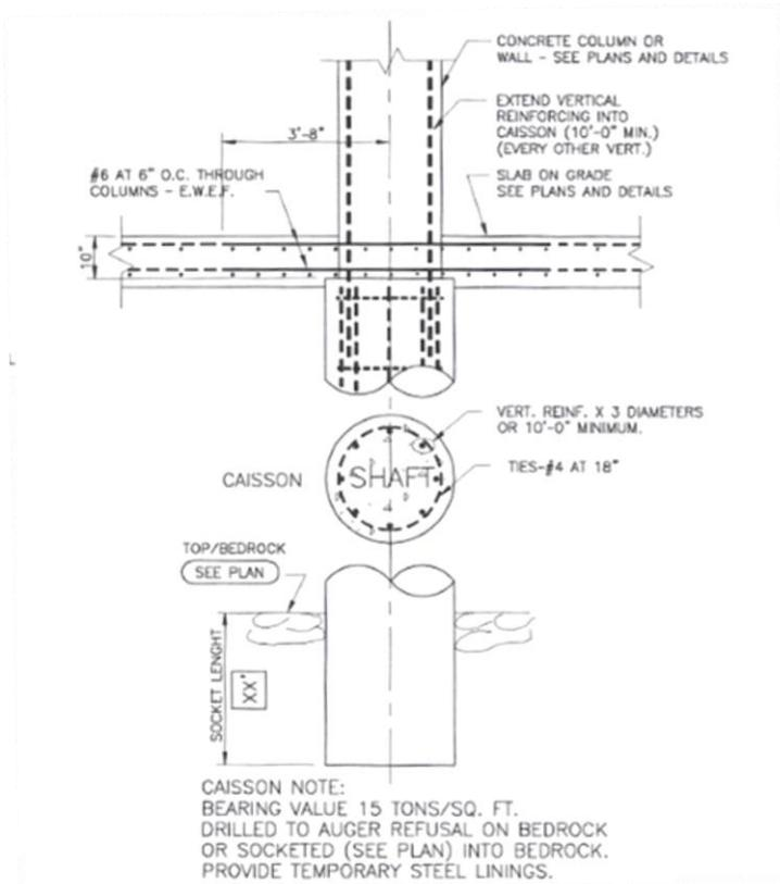
Figure 4- Caisson Detail
