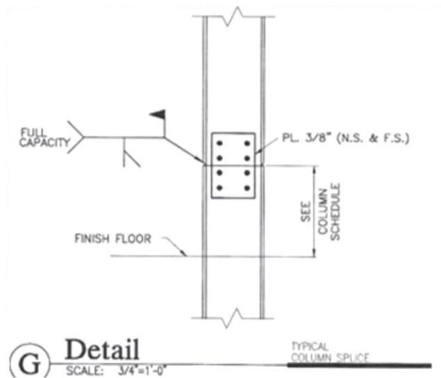
Figure 8- Splice Detail
