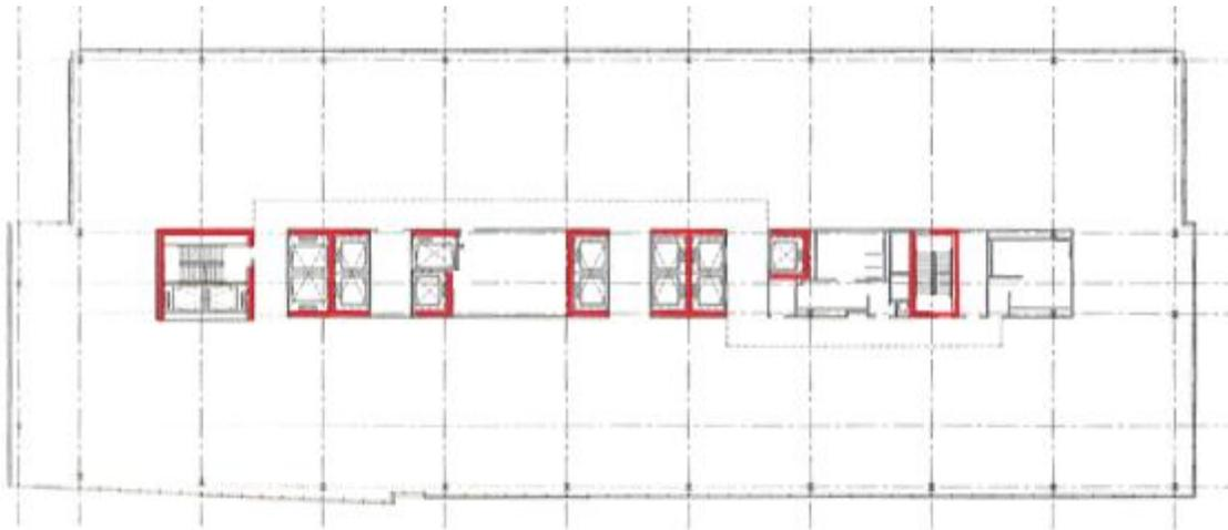
Figure 9- Shear Wall Layout
