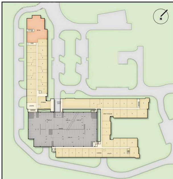
Figure 1: Site plan: Light Brown area represents the building. Gray area represents the parking garage. (Construction documents by Cates Engineering).
