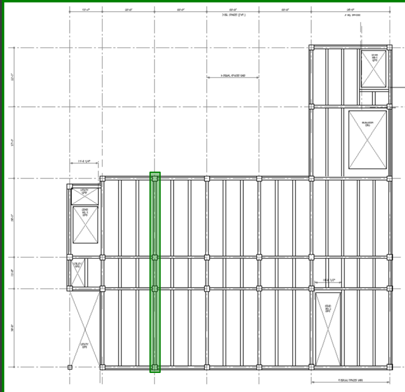
Concrete framing plan
