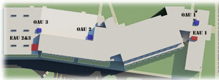
Figure 9: Air handler Layout on Second Floor Roof
