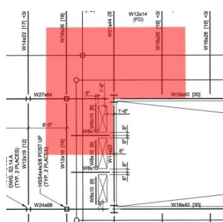
Figure 9 : C3 main roof tributary area
