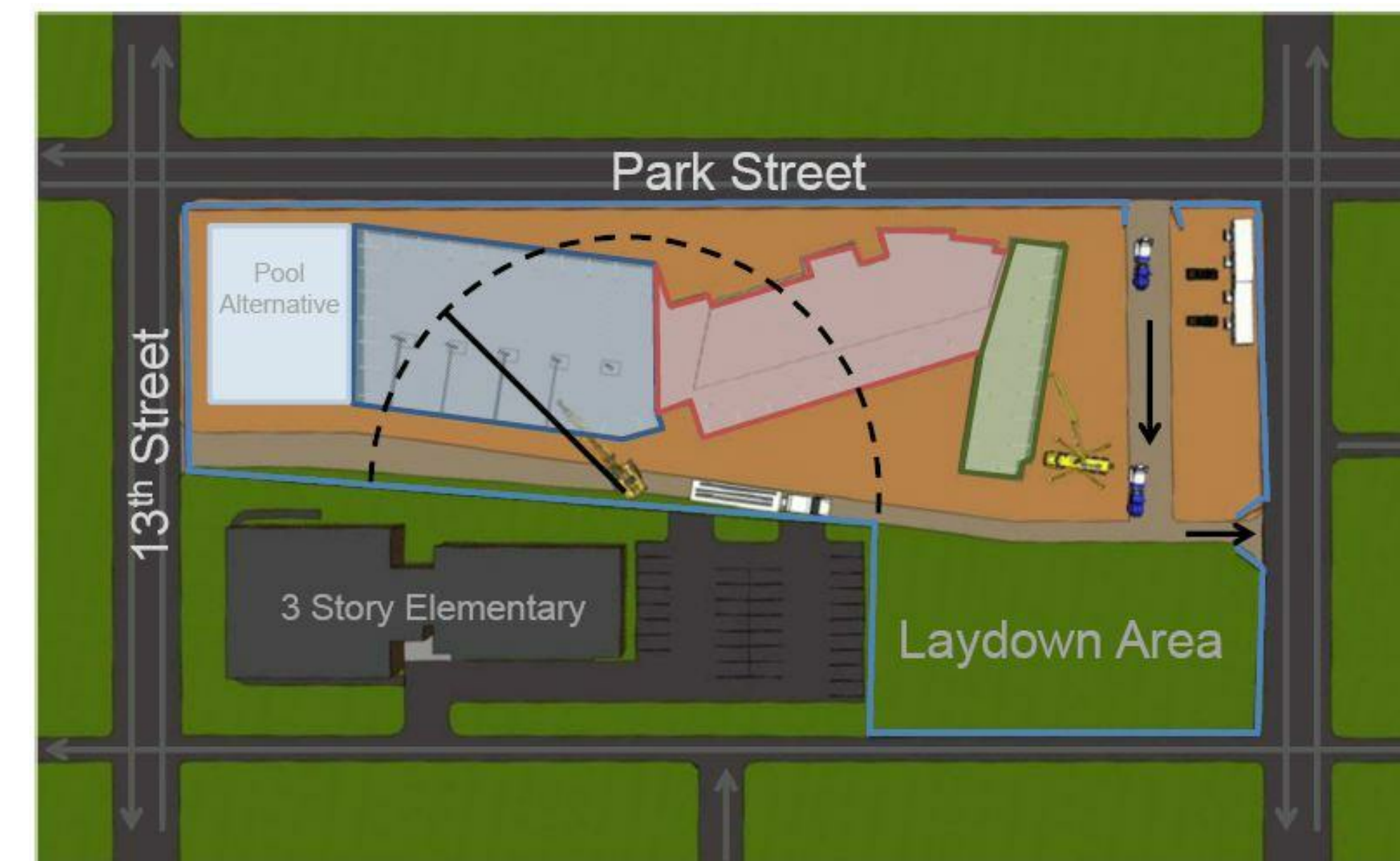
Superstructure Erection - 8/29/14 to 1/23/15
