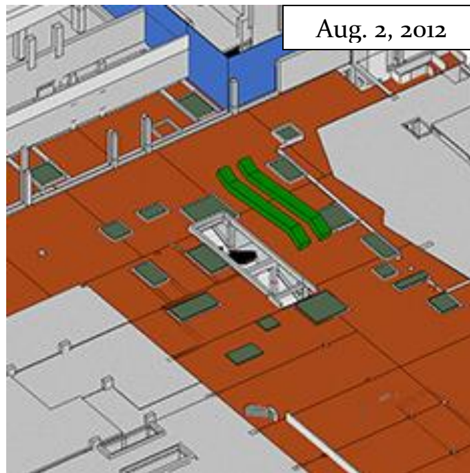
Figure 28: Original Intention of On Site Escalator Truss Storage
