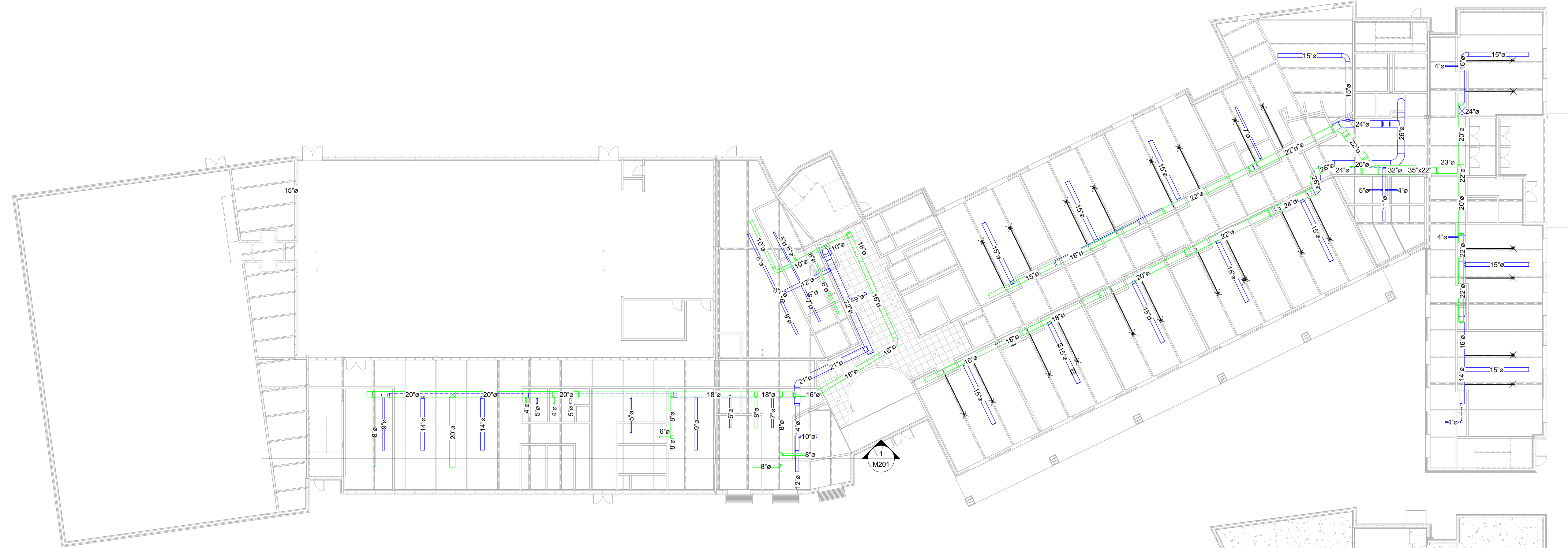
1 1st Floor Duct Layout 1/16" = 1'-0"
