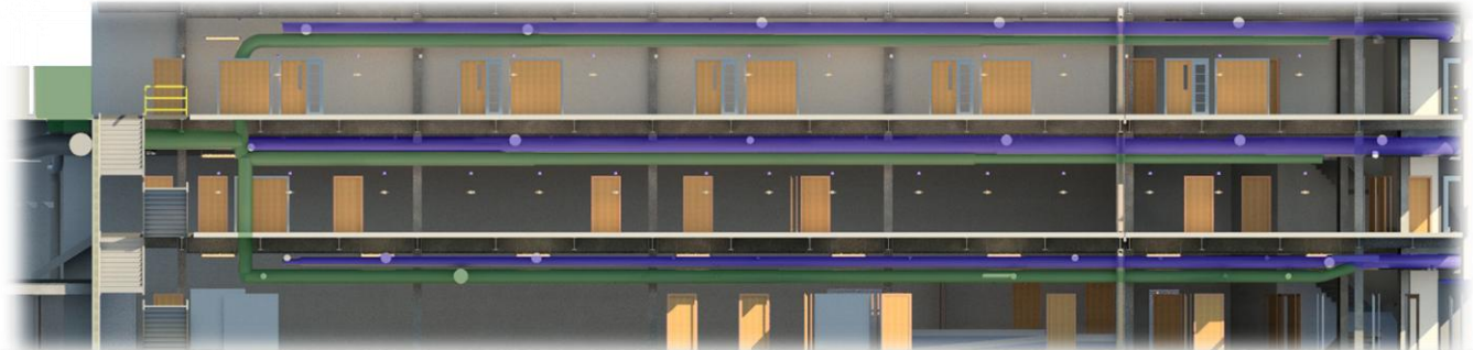
Figure 21: Section Rendering of West Wing Classrooms/Office Showing Configuration of Supply (Blue) & Exhaust (Green) Duct
