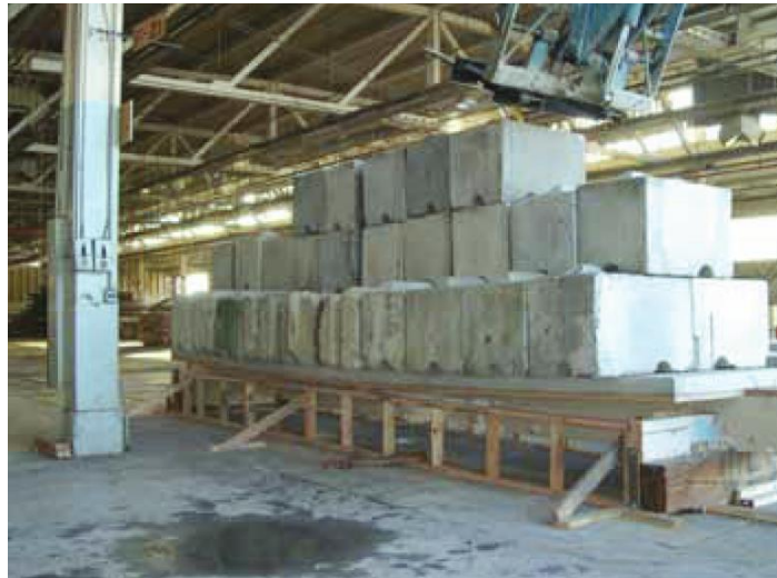
Figure 116: Tested beam before failure (Swenson et al.)
