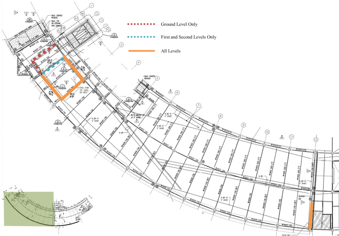
Figure 57: LFRS of west end of building
