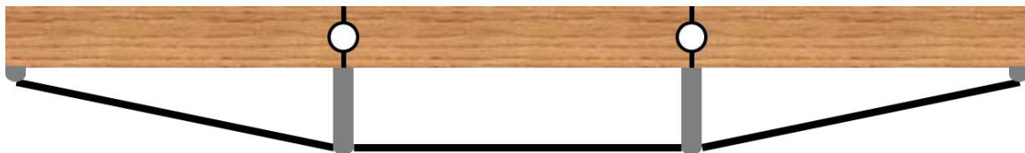
Figure 41: Simplified hinge queen post girder
