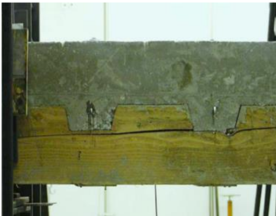
Figure 117: Shear failure of wood notch (Balogh et al.)
