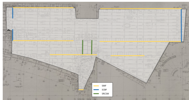
Figure 1.7: Locations of lateral force resisting elements in the patient bed tower
