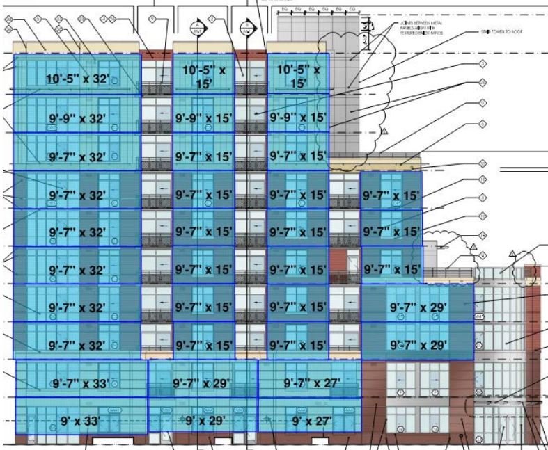
Figure 34: West Elevation Panel Breakdown
