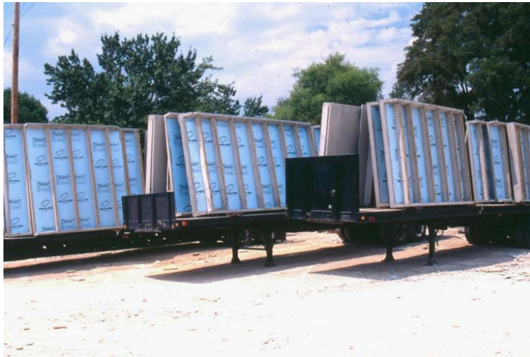
Figure 24: Transportation similar to Superior Walls ( http://www.superiorwalls.com )
