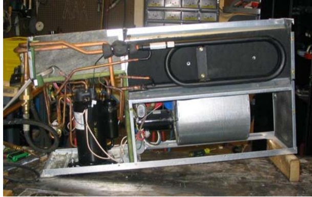
Figure I-7 A disassembled perimeter heat pump, heat pumps such as these control the interior envelope temperature and absorb most of the envelope heating load.
