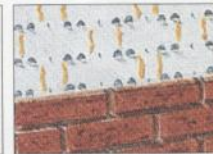
Metal tabs support the thin brick and assure straight, uniform bed joints.
