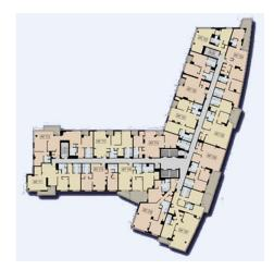
The Odyssey was designed through consideration of a minimum floor-to-floor height and an overall height limitation of 180' by the Code of Virginia zoning ordinances. The floor system must be designed per IBC 2003 International Building Code for the residential floors to resist all subjected dead loads and a live load of 40psf for residential space and 100psf for corridors. A list of relevant gravity loads follow:
