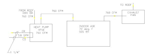
Rooftop heat pumps are used to condition the common areas throughout the building. The basic operation is the same as heat pumps located throughout the building with some minor differences. The rooftop location allows these heat pumps to be supplied directly from the outside without vertical supply ducts. Conditioned air is then supplied to the spaces below through vertical supply
