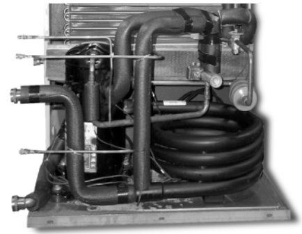
Figure 1: Coaxial heat exchanger
