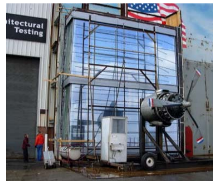
Figure 7 -Mock up of curtain wall system. (Photo courtesy of Gilbane).
