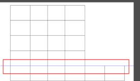
Parking Deck/First Floor: 4" Slab on 2" composite deck, W10x15 Beams, W24x76 Girders
