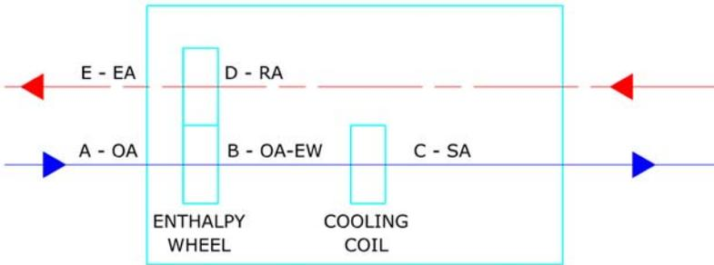
Figure 2.4B. DOAS Air Handling Unit State Points.
