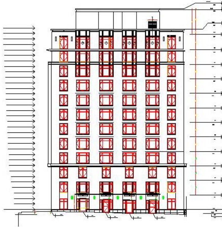
Wind loads applied to the North-South Direction
